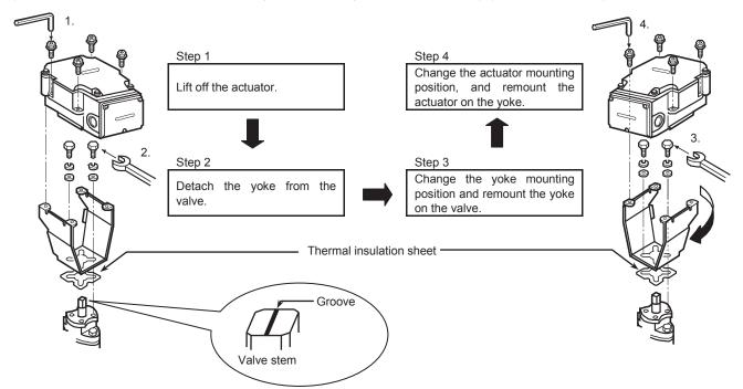
Figure 8. Changing the actuator mounting position
