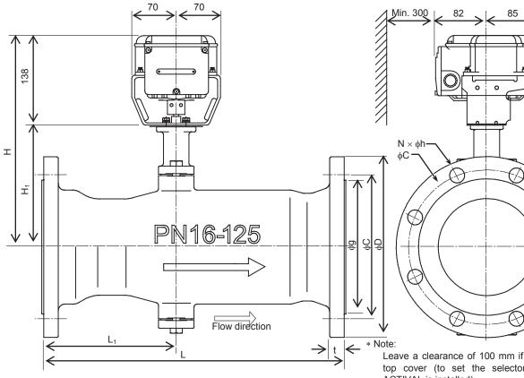
Leave a clearance of 100 mm if you do not open the top cover (to set the selector switches after the ACTIVAL is installed)
