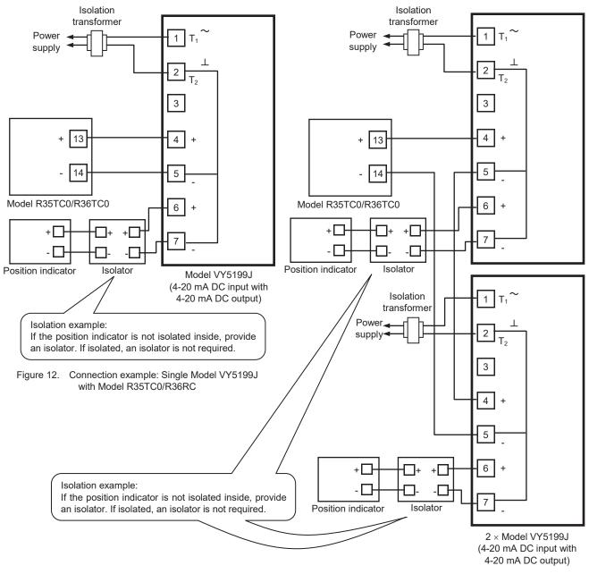
Figure 13. Connection example: Two Model VY5199J with Model R35TC0/R36RC (Parallel operation)
