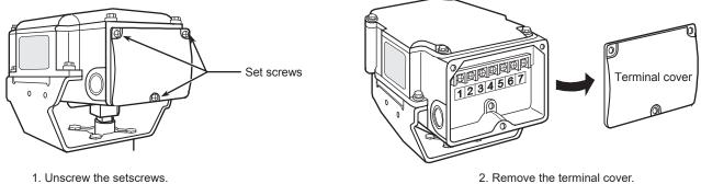
Figure 10. Terminal cover removal
