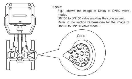
Figure 1. Mechanism of cavitation erosion resistance
