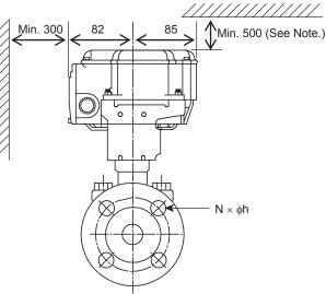
Leave a clearance of 100 mm if you do not open the top cover (to set the selector switches after the ACTIVAL is installed).
