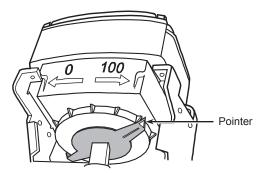
Figure 6. Preset pointer position for shipment
