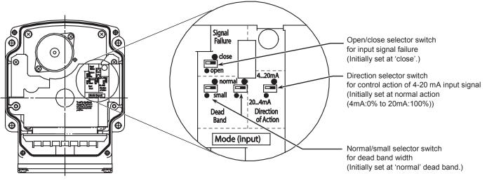
Figure 4. Selector switches
