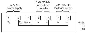
Terminals 2, 5, and 7 are connected inside the actuator.
