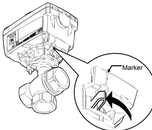
Figure 11. Locked position
