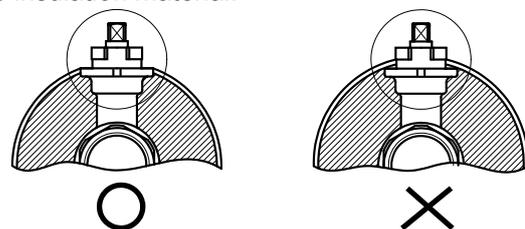
Figure 6. Heat insulating area
