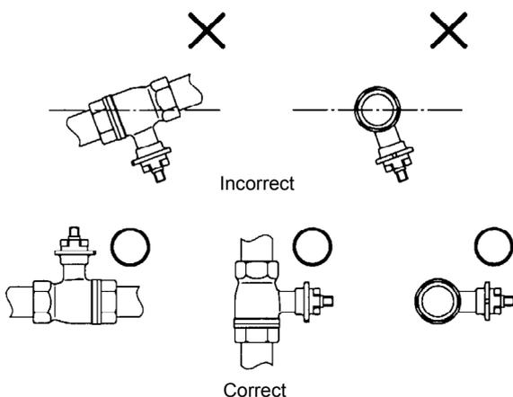
Figure 4. Mounting orientation
