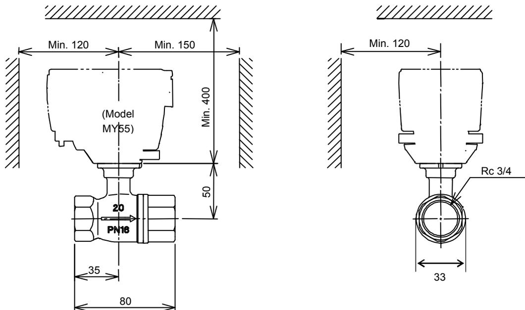
Figure 3. Actuator dimensions (mm)
