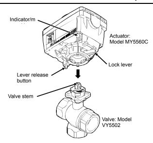
Note: Do not press the lever release button while operating. Keep the heat insulator away from the lever release button or the indicator/manual lever.
