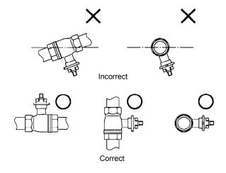
Figure 4. Mounting orientation
