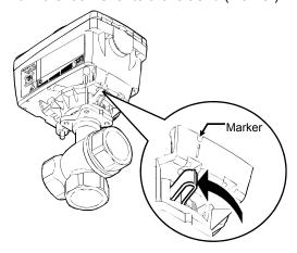
Figure 11. Locked position
