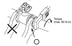
Figure 5. Attaching to pips
