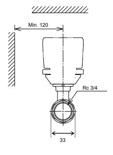
Figure 3. Actuator dimensions (mm)
