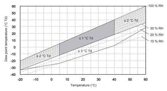
Figure 4. Duct sensor, dew point temperature accuracy (case ambient temperature: 25 °C)
