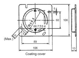
Dimensions of cover with JIS flange (unit: mm) (for medium size square box, commercial part)
