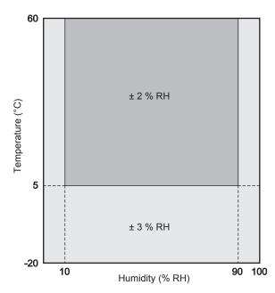
Figure 2. Duct sensor, humidity accuracy
