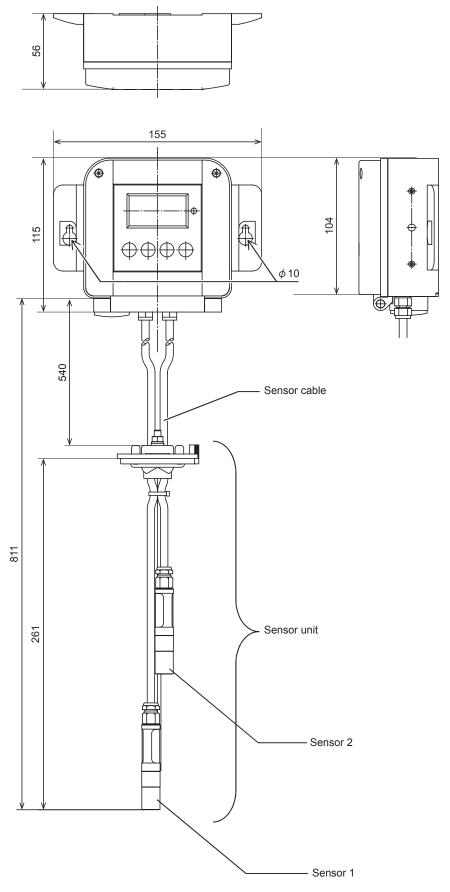
Figure 6. Duct sensor dimensions (unit: mm)
