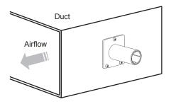
Figure 18. Attaching the mounting bracket
