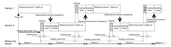
Figure 29. Basic operation after power ON (sensor 1 is in measuring mode)
