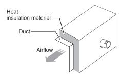
Figure 19. Heat insulating material installation
