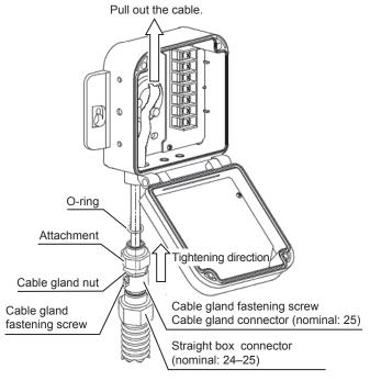
Figure 25. Cable gland attachment
