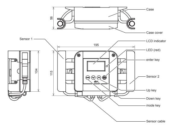
Figure 5. Indoor sensor dimensions (unit: mm)
