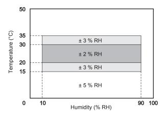
Figure 1. Indoor sensor, humidity accuracy
