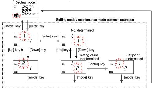
Figure 31. Operation mode transition diagram (in the setting mode)
