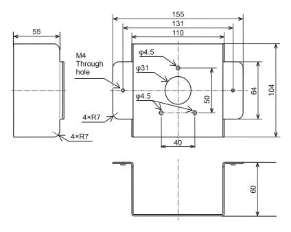
Figure 8. Main unit for duct mounting bracket dimensions (unit: mm)
