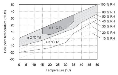
Figure 3. Indoor sensor, dew point temperature accuracy
