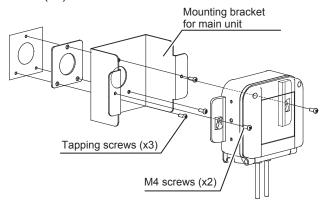
Figure 20. Attaching case
