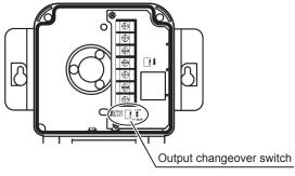
Figure 9. Output changeover switch (S1) position
