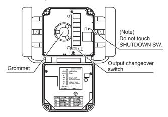
Figure 14. Position of grommet
