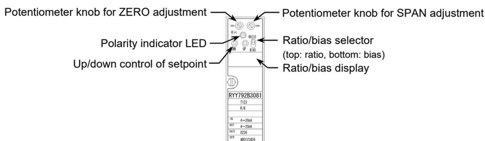
Figure 8. Front panel of the ratio bias
