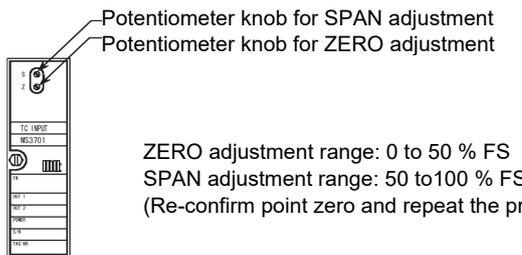
Figure 4. Front panel of the POT/I converter
