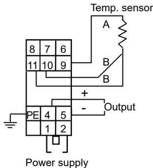
Figure 3-1. Connection diagram
