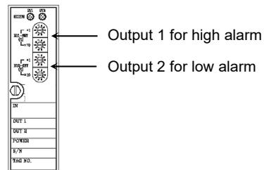
Figure 6. Front panel of the monitor switch
