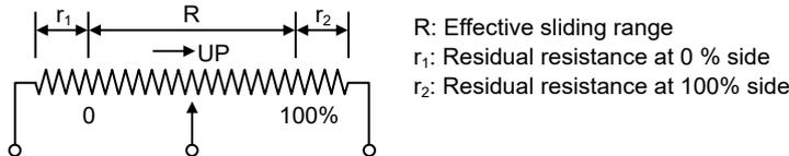
As the left figure shows, set the 0 % and 100 % points to make the residual resistances of the potentiometer be  $r_1 = r_2$ .
