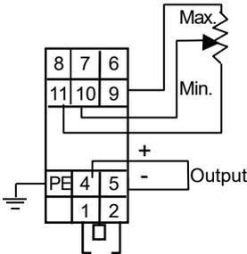
Figure 3-2. Connection diagram
