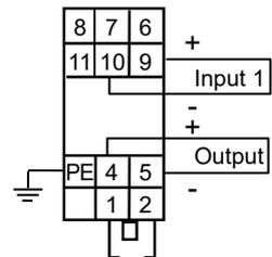
Figure 3-7. Connection diagram
