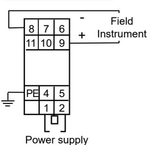
Figure 3-4. Connection diagram
