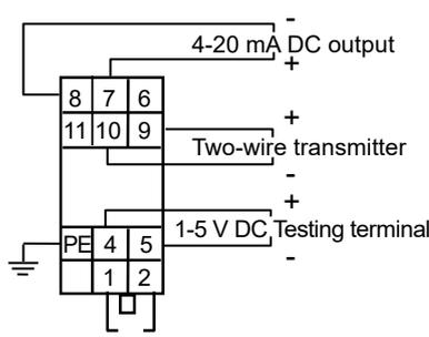
Figure 3-5. Connection diagram
