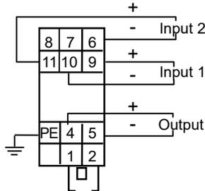
Figure 3-3. Connection diagram
