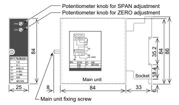
Figure 1. Dimensions (mm): With the socket assembled
