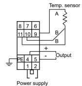
Figure 3-1. Connection diagram
