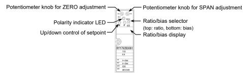
Figure 8. Front panel of the ratio bias
