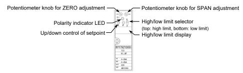
Figure 7. Front panel of the limiter
