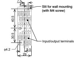
Figure 2. Dimensions (mm): Socket in front
