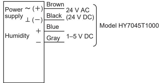
Figure 14. Wiring diagram (Room humidity sensor, 24 V AC/DC common power supply type)
