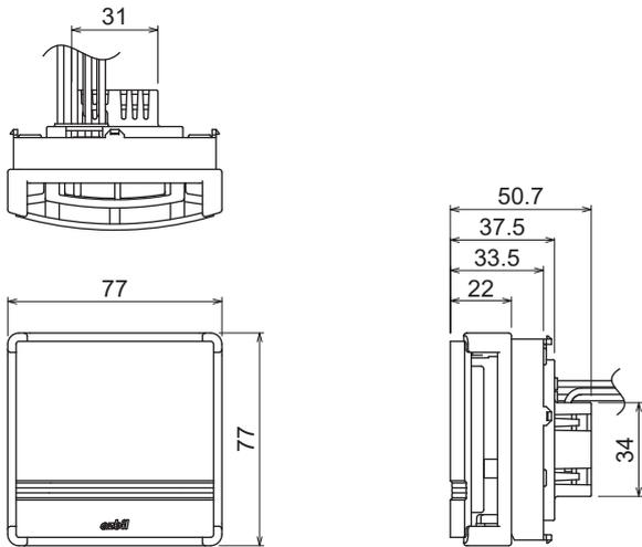
Figure 1. Main unit (mm)
