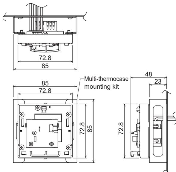
Figure 6. Dimensions when mounted in the Multi-thermocase mounting kit (mm)
