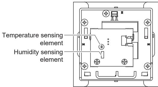
Note: The temperature/humidity sensor is illustrated as an example.
