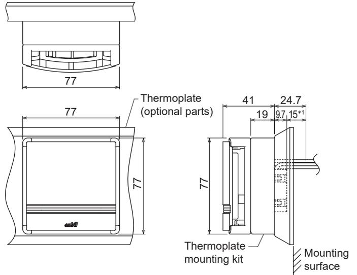
Figure 4. Dimensions when mounted on the Thermoplate mounting kit (mm)
