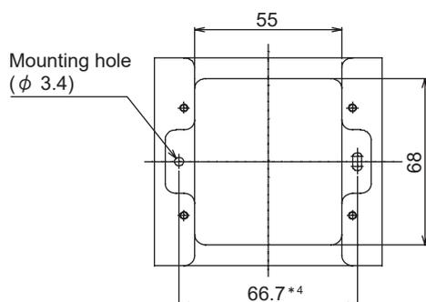
Figure 7. Surface of the Multi-thermocase mounting kit (mm)
