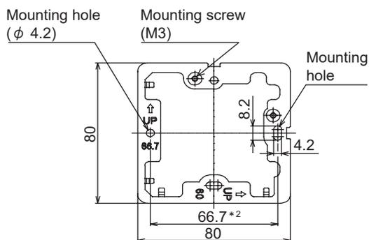
Figure 3. Surface of the mounting plate (mm)
