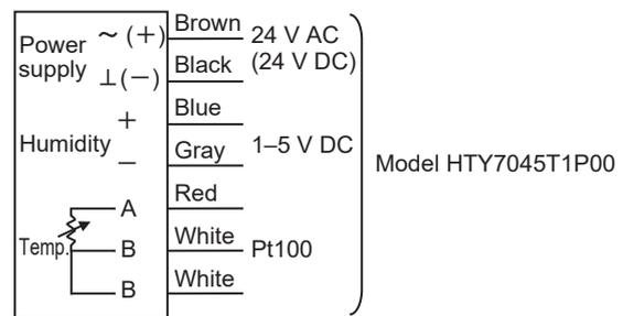
Figure 15. Wiring diagram (Room temperature/humidity sensor, 24 V AC/DC common power supply type)
