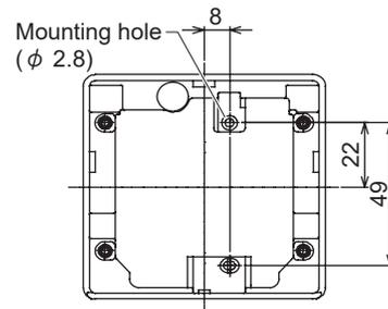
Figure 5. Surface of Thermoplate mounting kit (mm)
