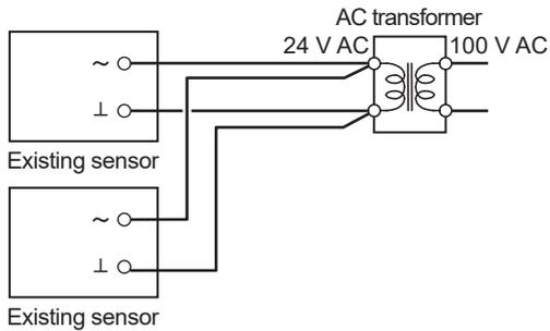
Figure 19. Wiring before replacement
