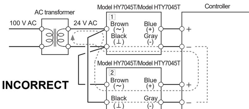
Figure 22. Incorrectly wired
