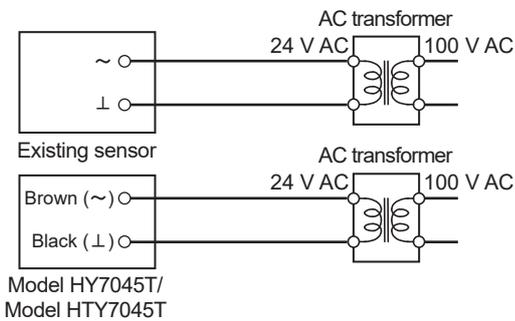
Figure 20. Wiring after replacement
