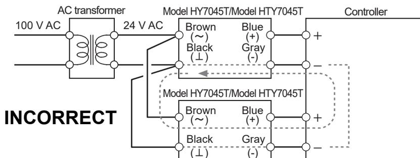
Figure 21. A loop is made in the circuit
