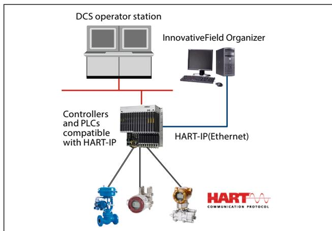
**Figure 12. IFO system configuration via HART-IP**
