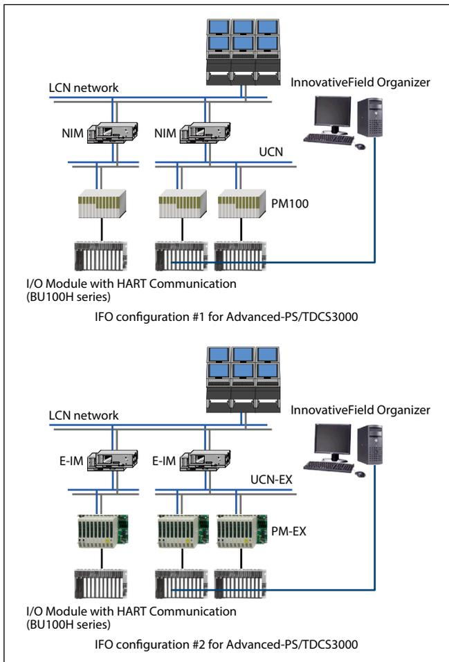
Figure 8. IFO Configuration for Advanced-PS/TDCS3000
