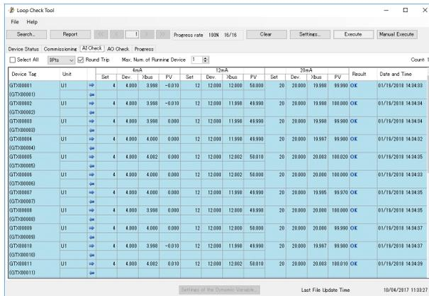
Figure 5. AI Check screen (while multiple devices are being checked)
