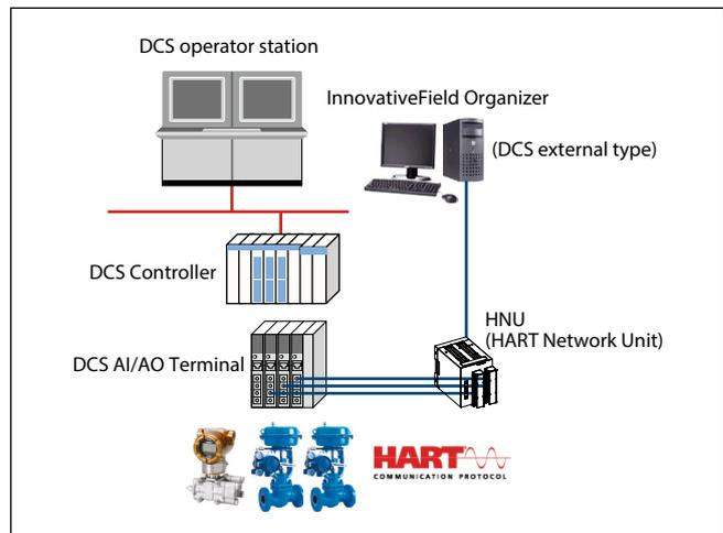
Figure 10. IFO system configuration which is independent from DCS
