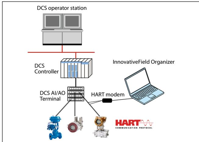
**Figure 11. IFO system configuration via a HART modem**
