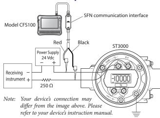
Figure 1. Example of SFN communication connection.
