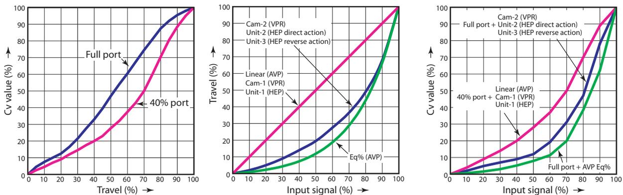
**a. Flow characteristics of valve    b. Positioner cam/unit characteristics    c. Modified flow characteristics**
