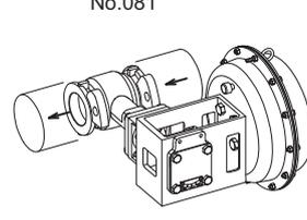
**Figure 6 Mounting position of valve on process pipes (Applicable to non-positioner case)**
