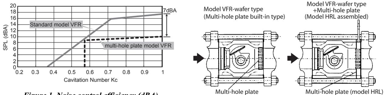
Figure 1 Noise control efficiency (dBA)
