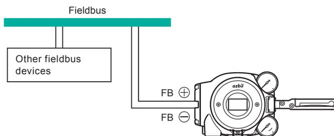
**Figure 2. Wiring example of AVP703**
