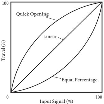
The graph plots Travel (%) on the y-axis (0 to 100) against Input Signal (%) on the x-axis (0 to 100). Three curves are shown: 'Quick Opening' (a curve that rises steeply at the beginning and then levels off), 'Linear' (a straight diagonal line from (0,0) to (100,100)), and 'Equal Percentage' (a curve that starts shallowly and becomes steeper as the input signal increases).
