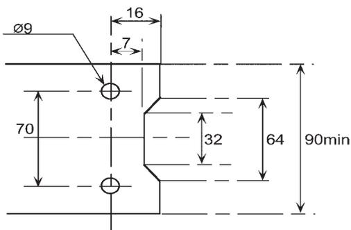
For single acting actuator with pressure regulator with filter
