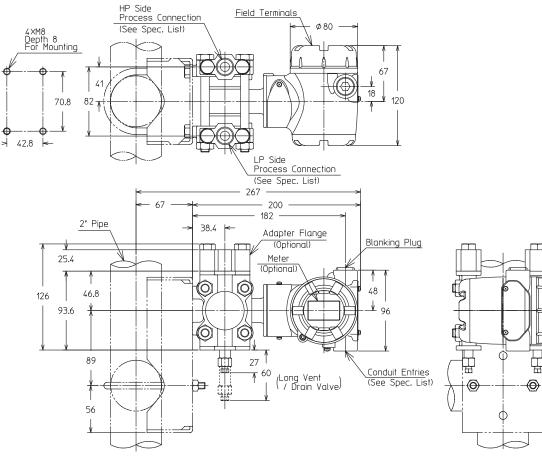
GTX 31D/41D (Material (Meter body cover, Vent/Drain plugs: PVC)
