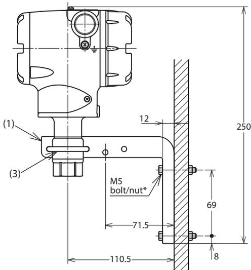
Note) \* Bolts for wall mounting are not included. (Length will vary according to wall thickness)
